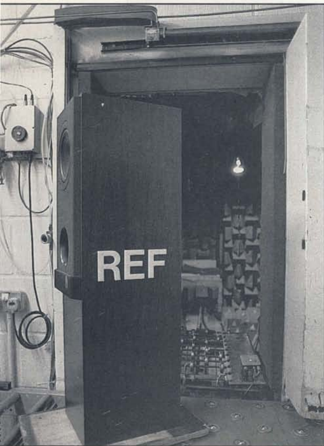
The Anechoic Chamber and the R103/4 Reference against which production models are checked.
