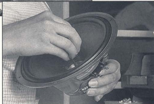
Above: Inserting the tweeter into a 'Uni-Q' drive unit.
