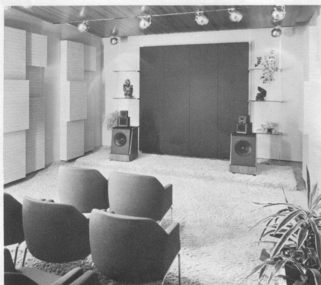
Fig. 11. Listening room for subjective checking. The sound absorption units on the walls and ceiling are designed to provide ideal listening conditions.
