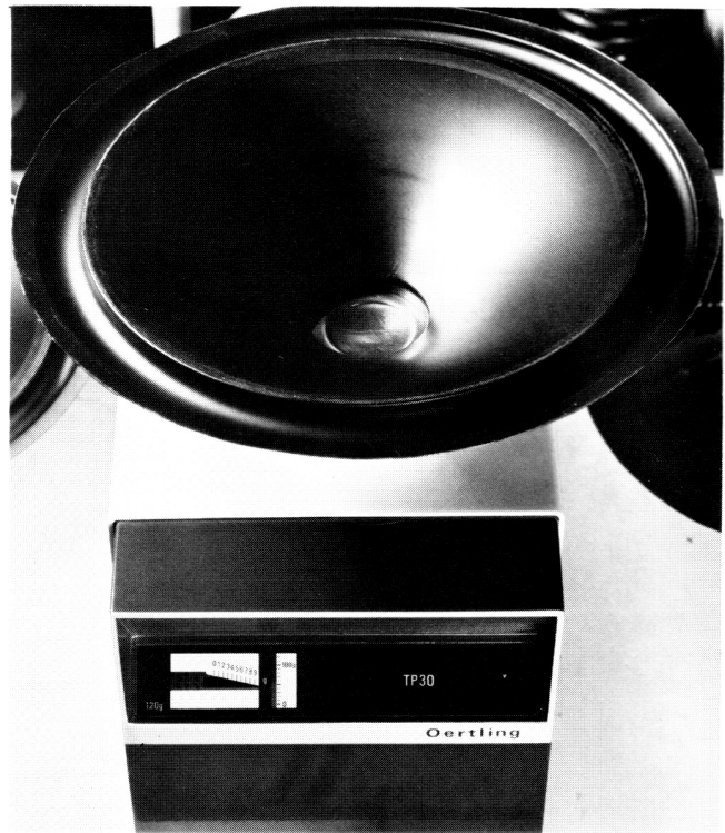
Fig. 1. Weighing diaphragms to check the thickness of the visco-elastic damping layer; the balance is sensitive to changes of 10 milligrams.
