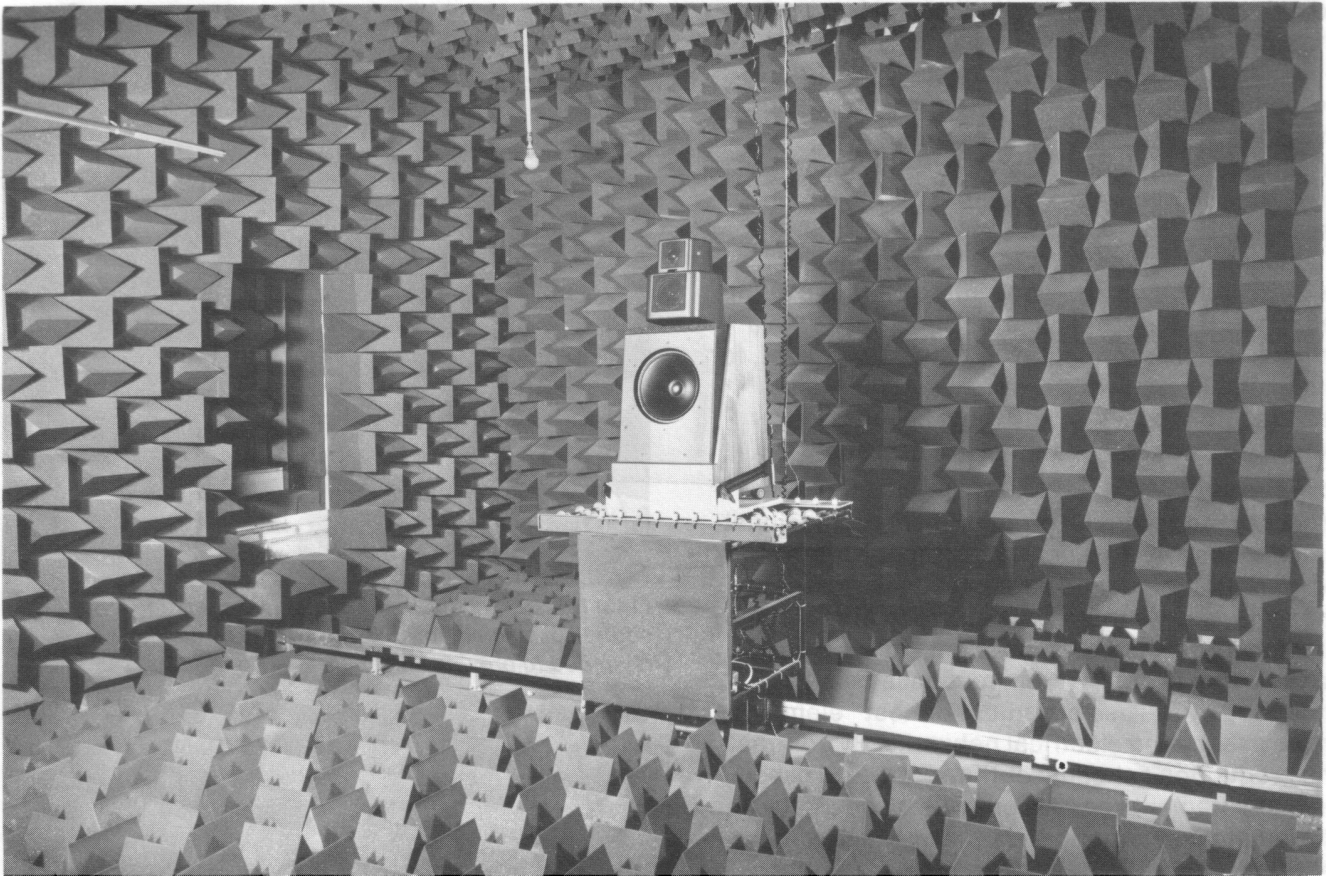
Fig. 9. System test chamber for head assemblies and complete loudspeakers.
